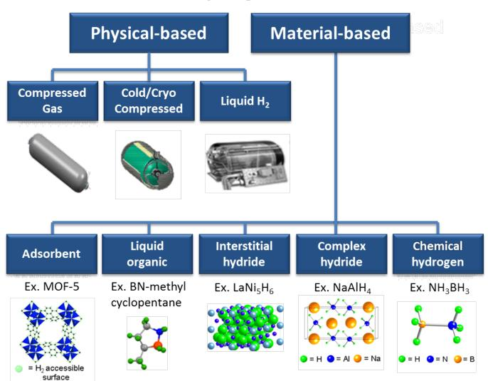
Hydrogen can be stored physically as either a gas or a liquid. Storage of hydrogen as a gas typically requires high-pressure tanks (350–700 bar [5,000–10,000 psi] tank pressure). Storage of hydrogen as a liquid requires cryogenic temperatures because the boiling point of hydrogen at one atmosphere pressure is -252.8°C. Hydrogen can also be stored on the surfaces of solids (by adsorption) or within solids (by absorption).
