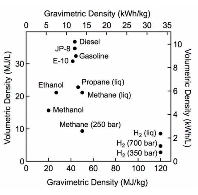
O Comparison of specific energy (energy per mass or gravimetric density) and energy density (energy per volume or volumetric density) for several fuels based on lower heating values.
